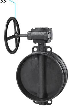
The Model B333 Large Diameter Butterfly Valve provides efficient control of fluid flow in piping systems. It is a grooved-end bubble tight shut-off valve with end-to-end dimensions that meet MSS SP-67, Table 4 and a mounting pad that meets ISO 5211 for the mounting of power actuators. The valve is capable of bidirectional fluid flow at working pressures to 300 psi (20 bar) and may be positioned in any orientation.
